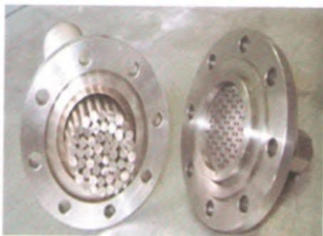
Figure 5. Cobaltic chloride filter elements.
